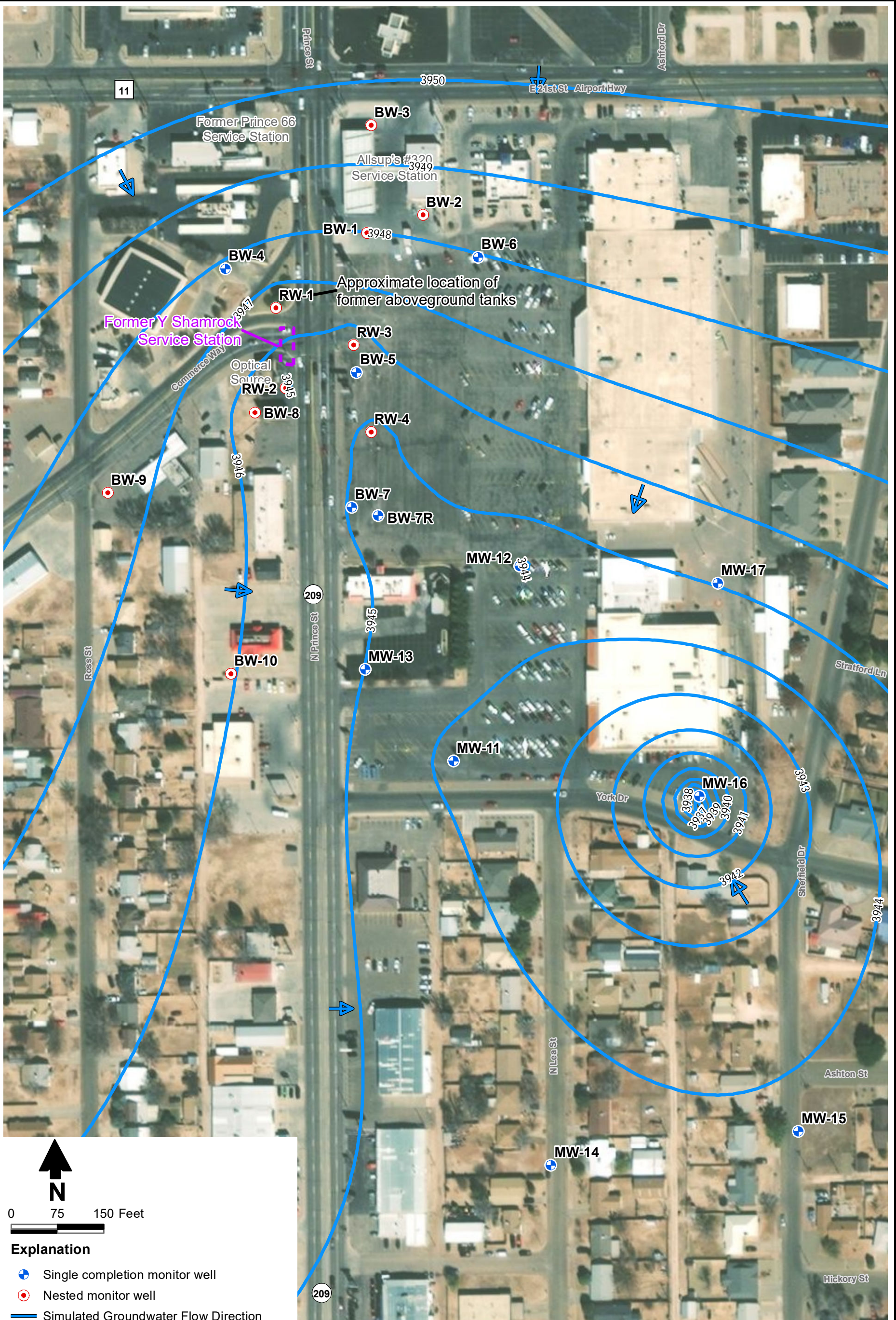
FORMER Y STATION STATE LEAD SITE CLOVIS, NEW MEXICO Minimum Pumping Scenario Groundwater Elevation Contour Map: 5 Year Simulation
